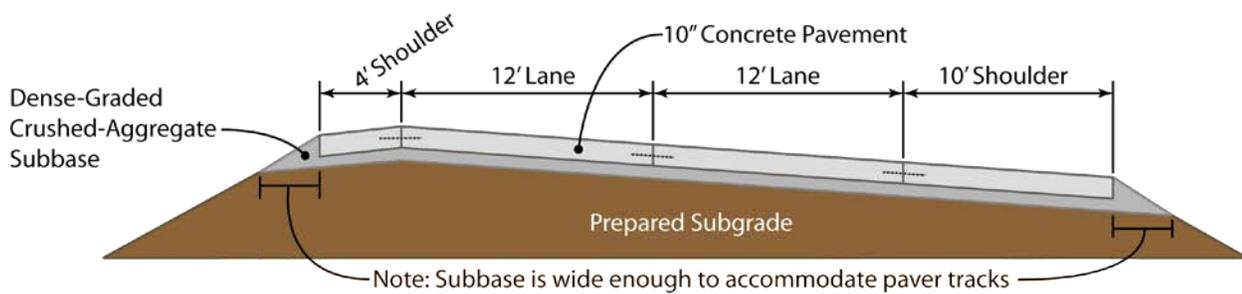
**Figure 1 Cross Section of "Standard" Construction Project**
