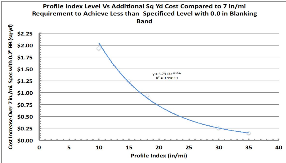
Figure 14 PI with 0" Blanking Band Versus Additional Cost to Achieve the Specified Roughness Compared to the Cost to Achieve 7 in./mi. PI with 0.2" Blanking Band
