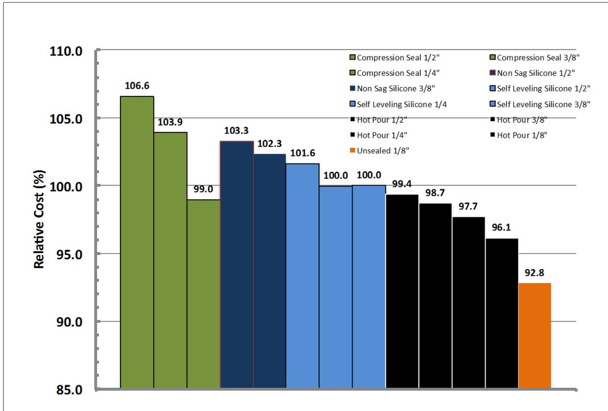
Figure 12 Relative Cost of Sealant Installations by Product Type
