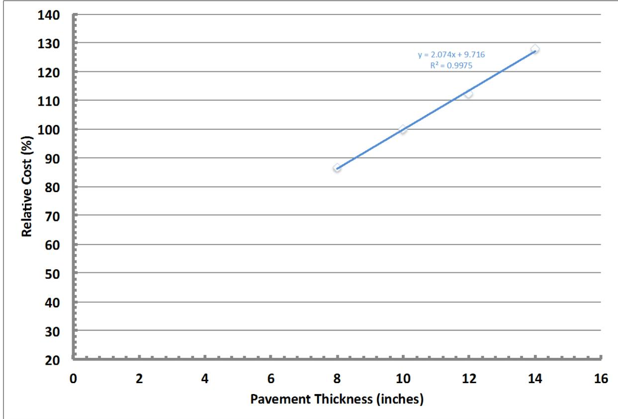
**Figure 4 PCCP Thickness Versus In-Place Construction Costs**
