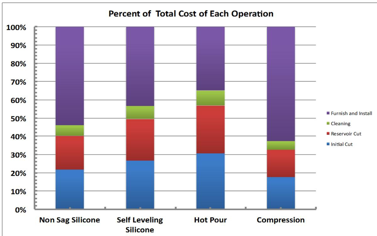
Figure 11 Percent of Total Installation Cost of Each Sealant Construction Phase
